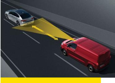
Forward Collision Alert¹: scans the road ahead to alert the driver to the potential for a collision with vehicles or pedestrians. Additionally, the Semi-adaptive Cruise Control¹ lowers your speed to maintain a set distance to the car ahead in traffic scenarios and restores your previous speed when the road clears.
