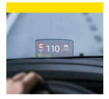
Head-up Display: unique in the segment to the Vivaro, see vital info such as speed and Semi-adaptive Cruise Control data projected in the driver's line of sight on the Head-up Display<sup>2</sup>.
