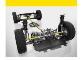
**4x4 conversion**<sup>1</sup>: choose the Dangel 4x4 conversion for highly capable mobility on challenging road surfaces or even rugged offroad terrain. Additionally a 4x2 conversion is also available from Dangel.
