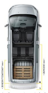
Load space: an impressive load length (on floor) of up to 2,36 m and a maximum load height of 1,39 m.
