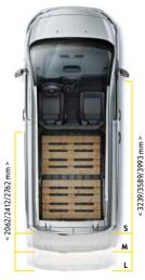
Available in 3 sizes of body length—Small, Medium and Large—the Vivaro perfectly adapts to your business needs, each variant offering a balance between relatively compact exterior dimensions and a spacious, flexible interior. The Small version in particular, at just 4,60 m in length, is perfectly agile in tight city streets and urban areas where space is limited. This variant can load 2 euro-pallets, while the Medium version can comfortably carry 3 euro-pallets.
