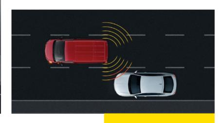
**Side Blind Spot Alert**<sup>1</sup>: uses sensors and a visual projection on the wing mirror, alerting the driver to vehicles in the Vivaro's blind spot to prevent accidents in overtaking situations.
