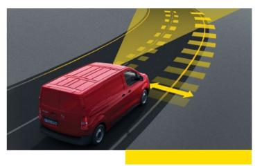
Lane Departure Warning<sup>1</sup>: recognizes when the Vivaro is drifting lanes and alerts the driver via audio and visual cue.
