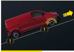
Hill Climb Assist': keeps the car from rolling backwards when stopped on an incline and holds the brake for you while you switch from the brake pedal to the gas pedal.
